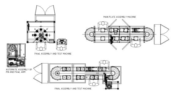
This engineering project covered the supply of a suite of special assembly machines for an industrial automation cell. The automated production line consisted of four machines to automatically assemble and function test an automotive seat recliner mechanism.
